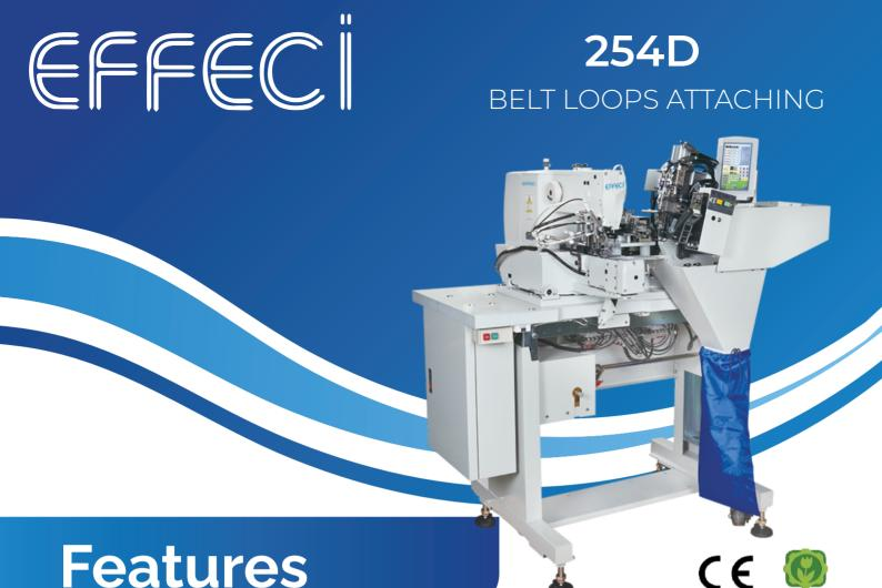
Automatic two-needle unit for attaching belt loops to denim trousers and classic trousers. The machine automatically proceeds to cut the belt loop, fold it and sew the reinforcing bartack to the jeans. Automatic position detection and removal of the belt joint as waste material. The automatic unit improves efficiency by 70% compared to 4 operators with the classic method.
